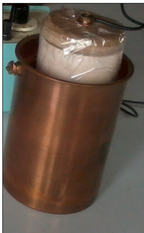
Fig. 5: DC-MFC using Porous Pot
